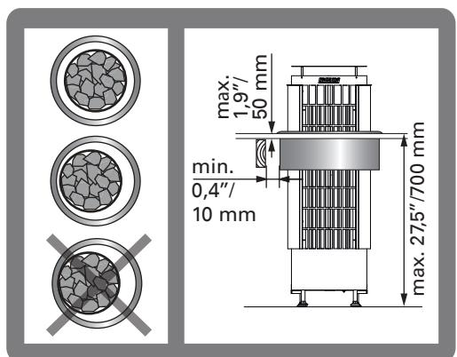
**NOTE!** The benches' distance from the heater can be less than specified in the heater's installation instructions when Harvia HPC2/HPC7 embedding flange is used. See also heater's instructions for installation.
