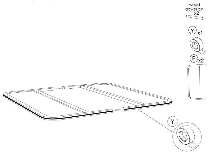
**STEP 7**: Draw a line on the center stave where the middle is. Take one of the panels (F) and put it directly next to the middle line. Fix it at the panel threshold with screws (S2). Pre-drill holes in the panel threshold, evenly spaced and not too close to the sides. Connect both panels with (C) stave, front and back, and fix using screws (S10). Make sure it's leveled.
