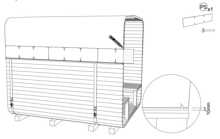
**STEP 31:** For 1st shingle cut off the half of hexagonal part. Remove protective film from the bottom of the sheet. Start placing shingles over starting shingles. Fix 2nd shingle next to first. 3rd shingle needs to be cut. Measure the necessary length and fix it with nails.
