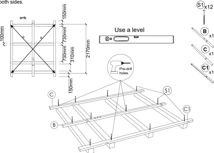
**STEP 2:** Fix 9 staves (C; C1) to each side from the center stave. Check level while installing staves and use rubber hammer for tighter placement. Pre-drill holes for screws. Use spray foam between boards for better insulation. After 9 staves are fixed, take of side staves and fix them.
