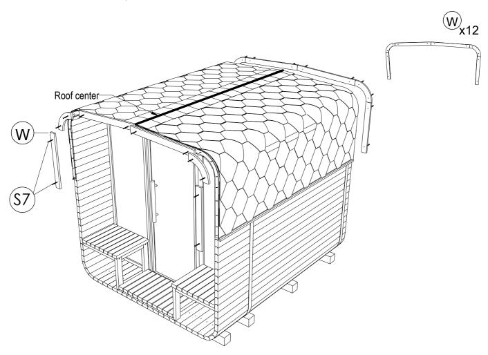
**STEP 38:** Use bitumen sealant behind decorative boards to fill gap between shingles and boards at the front and back side.
