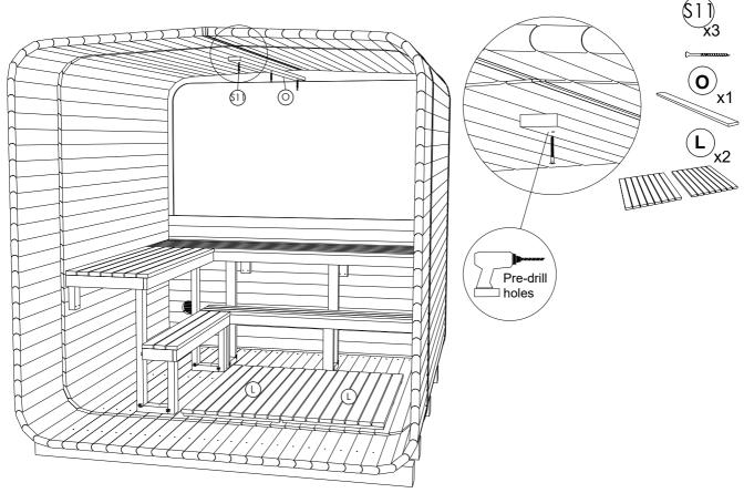
**STEP 25**: Fix the backrest (J2) in front of the panoramic window 150mm up from the sauna bench. Then install backrest staves (J6) at the same height as (J2).Pre-drill holes for screws.
