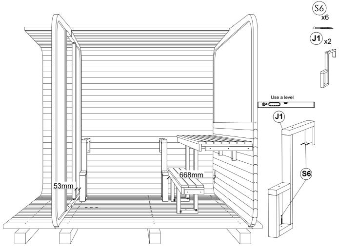
**STEP 23**: Fix sauna bench (J4) on top of the legs (J6) using (S6). Bench cross boards have to match the tops of the bench legs. Fix Bench step (J7) using (S6) screws.
