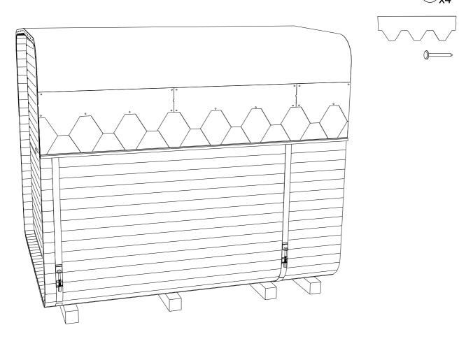
**STEP 33:** Third row goes exactly like first row. Cut half of hexagonal part from shingle and fix it with shingle nails. Remove protective film from the bottom of the sheet.  $(P1)_{VA}$
