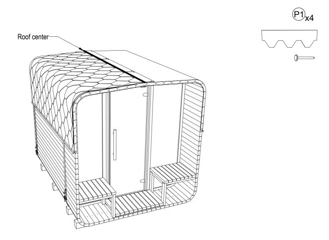
**STEP 35:** Repeat same steps for other side, till last layer goes over middle of the roof. Use heat source for better adhesion. Lift every rectangle, heat a bit and press it to the roof.
