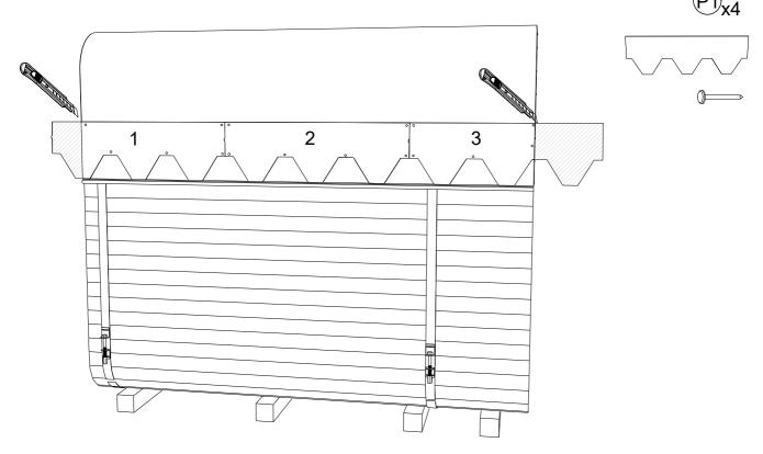
**STEP 32:** Remove the protective film from the bottom of the sheet. The second row starts with the whole shingle, fix it with shingle nails. Last shingle needs to be cut by measured length.
