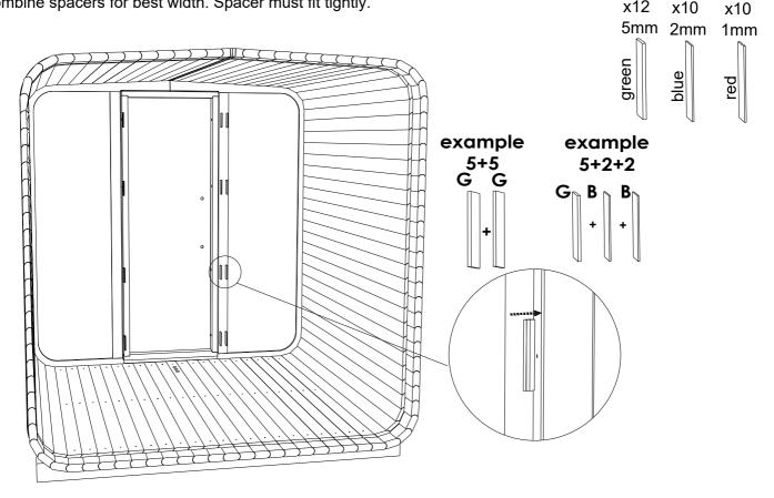
**STEP 18:** Fix one side of the door box with screws (S14) slightly to the outside through spacers. Then put spacers in other side. Combine spacers for necessary width. Spacers must fit tightly, they can't slip down before door is fixed with screws. Use screws (S14) to fix doors. Check door box, both sides should be straight, they must not be bent inwards or outwards.
