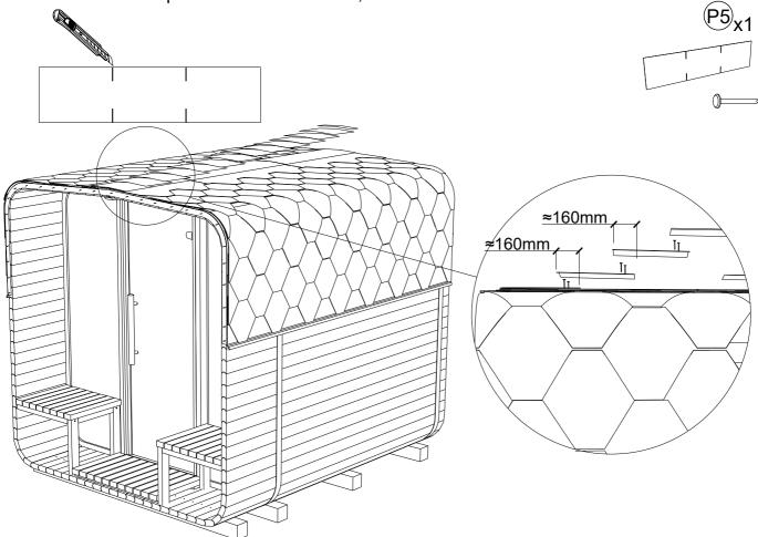
**STEP 37:** Install front and back decorative roof finishing boards using (S7). Start by fixing two top boards, then rest of it goes next to each other.
