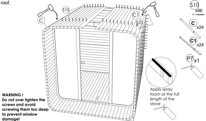
**STEP 13**: Finish roof with (C; C1) staves and final staves (H). If needed, use thinner staves (H1) to fil the gap between (H) staves and apply spray foam between staves. Make sure that centre of the roof is tightly filled, then fix with screws (S10).
