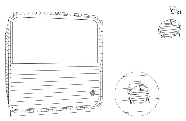
**STEP 15**:Install metal bands over the screw heads. **Screws (S9) must be placed as shown in picture**, then tighten the screws. Check the bands align evenly all around the sauna 95-100mm from the back and 495-500mm from front. Keep tightening bands till you feel strong resistance, bands can't be loose. Re-tighten the bands after a few days.
