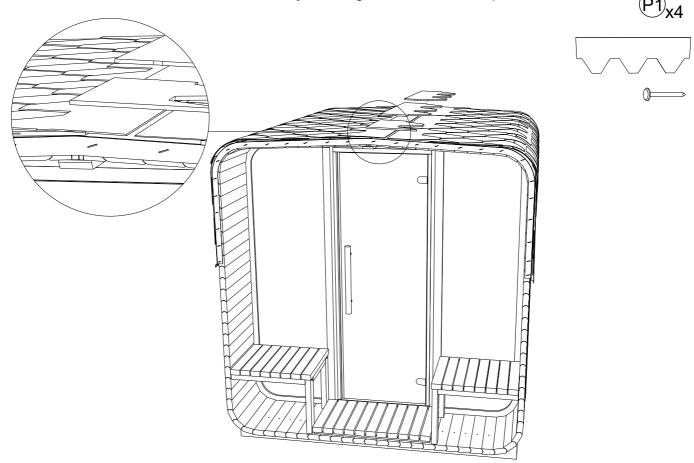
**STEP 36:** For top of the roof use starting shingles. Cut some shingles in squares, there are marked lines. Take off protective film. Nail each shingle with two nails. Next shingle goes about 160mm over previous. After it's done, use heat source for better adhesion.
