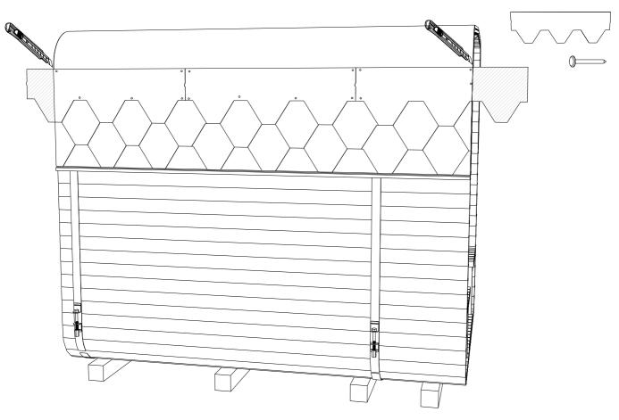
STEP 34: Keep placing shingles till last layer goes over the middle of the roof.
