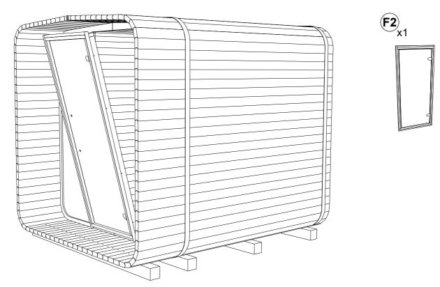
**STEP 17:** Put plastic spacers in the gap between the door box and the front panel where the screws go. Combine spacers for best width. Spacer must fit tightly.  $x_{10}$
