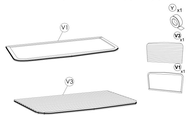
**STEP 11**:Install the panoramic panel (V1)or panel (V3) with caution. Use spray foam between panels for better insulation. Place it on top of the lower back panel (V). Check level and that side edges are aligned with bottom panel. One keeps holding the panel, and the other is fixing the side stave on a upper curve using screws (S10). Secure the panel (V1;V3) at the both
