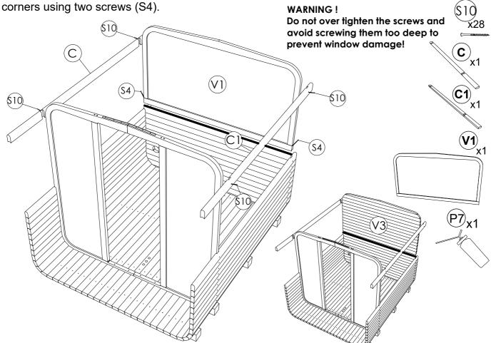
**STEP 12**: Fix 24 staves (C; C1) on both sides with screws (S10). Use rubber hammer for tighter placement. Use spray foam between every stave. Keep fixing staves till reach top of the
