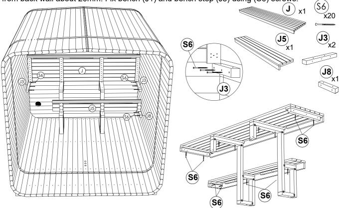
**STEP 22**: Install bench legs (J6) with (S6) screws. Take measurements as in the picture. Check the legs to ensure they are straight from all angles.
