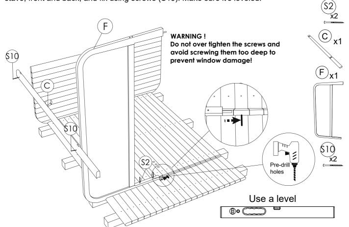
**STEP 8**: Place the second front panel (F). Slide it together that the top and bottom connects. Fix it at the panel threshold with screws (S2) pre-drill holes. Make sure it's level. Use metal bracket
