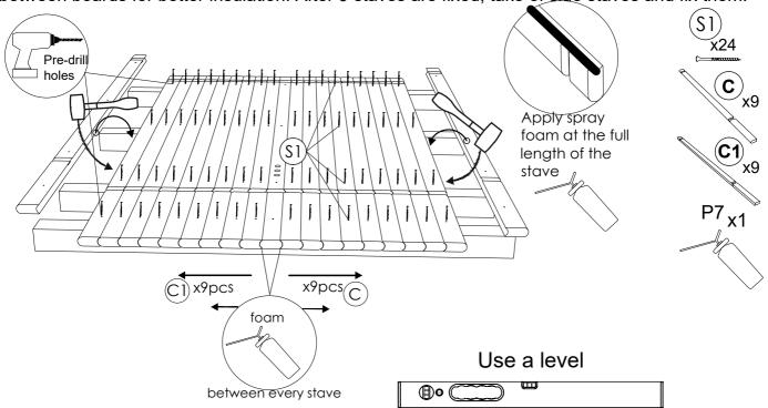
**STEP3:** Drill twenty 10mm holes in front and back wall groove to the out-side in board connections as shown in the picture. This will help drain excess water faster.
