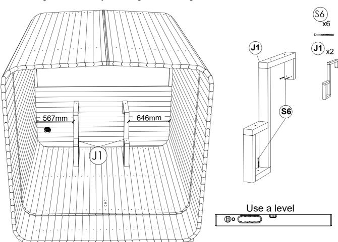
**STEP 21:** Place long sauna bench upwards on the bench legs. Then install bench support boards (J3) on the side walls using S6 screws, at the same level as the bench legs. Leave gap from back wall about 20mm. Fix bench (J1) and bench step (J5) using (S6) screws.
