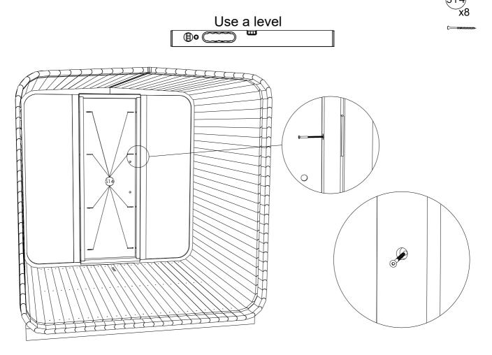
**STEP 19:** Use spray foam around door box. Let the spray foam dry. The excess amount will come off easily if you don't touch it while it's wet. Fix door moldings to both sides and on top of the door with (S11) screws.
