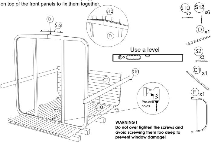
**STEP 9**: Fix 12 staves (C; C1) on both sides with screws (S10). Use rubber hammer for tighter placement. Use spray foam between every stave. Keep fixing staves till reach top of the rear panel (V).
